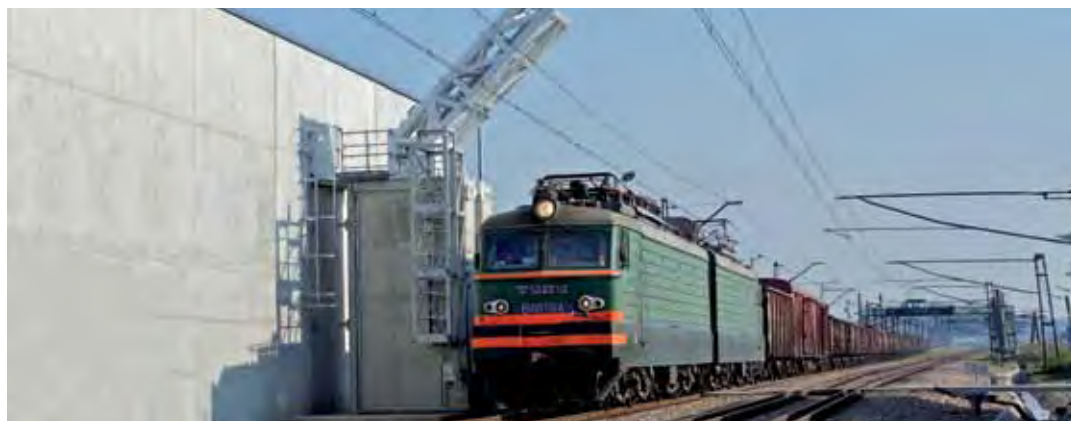
New scanner used to inspect rail wagons at the rail crossing point between Ukraine and Poland.
